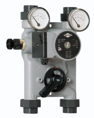
The WITA Bloc T 60 is a compact fitting made of grey cast iron that combines the circulating pump, mixer and, if requested, overflow valve in a single casing. It is primarily designed for smaller and medium-sized warm water heating systems. Because of the rotational direction of the pump, the supply direction is to the right.
